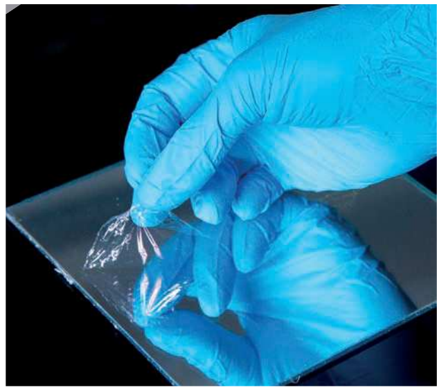
Parylene peeled-off from a mirror
