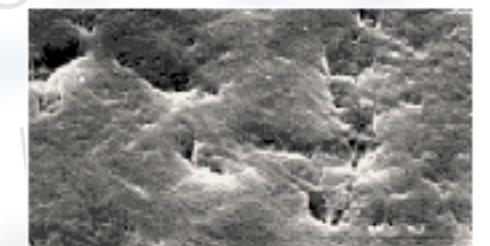
PTFE surface: before plasma treatment
