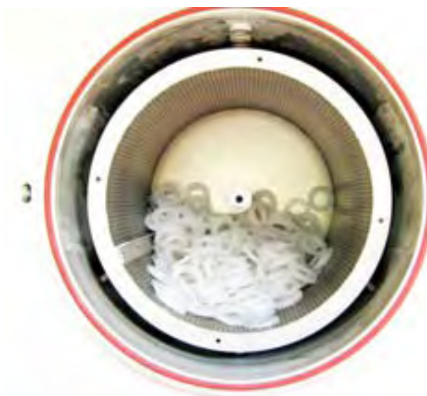
fig. 125: rotary drum for Nano (open, built-in)
