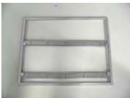
fig. 148: carrier for leadframes
