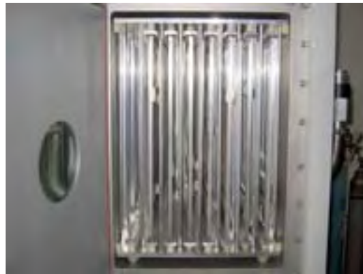
fig. 143: TETRA-150, special electrode for pcb
