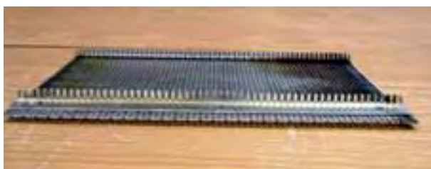
fig. 146: carrier for Leadframes
