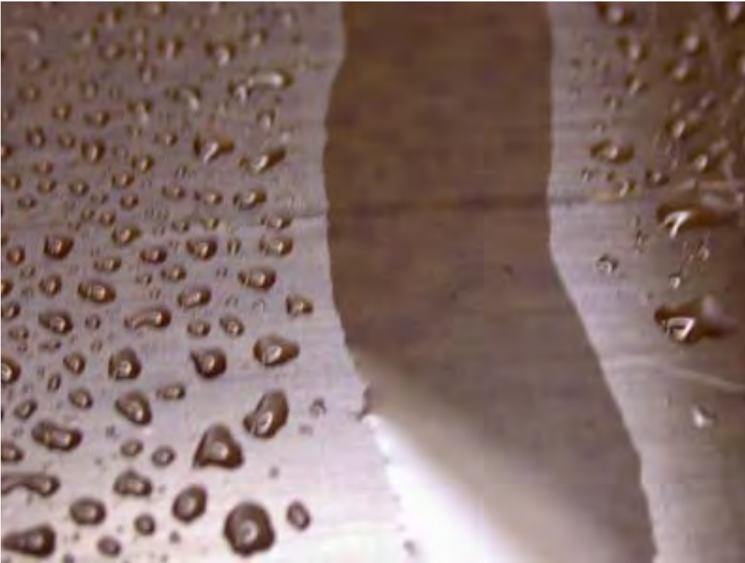
fig. 165: difference: plastics with and without plasma treatment
