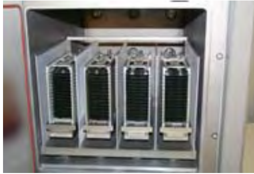
fig. 141: TETRA-30, electrode for leadframes
